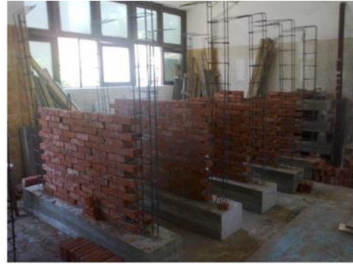
(b) Brick Wall Construction
